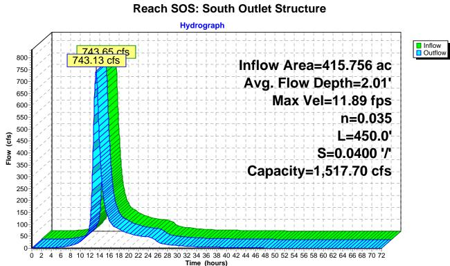
JEC Inactive Pond - Closure Inflow Design FloodType II 24-hr 100-yr, 24-hr Rainfall=7.44"Prepared by Aptim Environmental & Infrastructure, Inc.Printed 4/16/2018HydroCAD® 10.00-15 s/n 04891 © 2015 HydroCAD Software Solutions LLCPage 12
