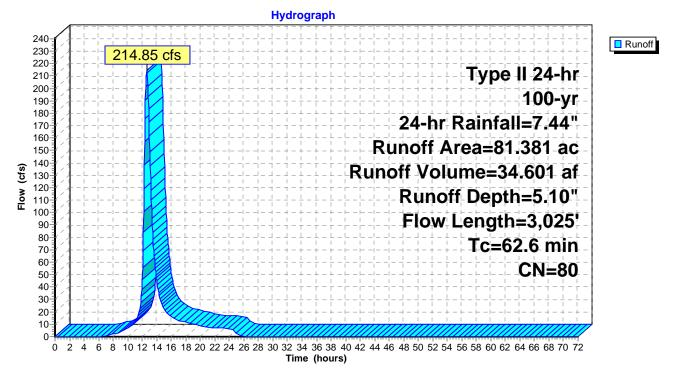
JEC Inactive Pond - Closure Inflow Design FloodType II 24-hr 100-yr, 24-hr Rainfall=7.44"Prepared by Aptim Environmental & Infrastructure, Inc.Printed 4/16/2018HydroCAD® 10.00-15 s/n 04891 © 2015 HydroCAD Software Solutions LLCPage 6
