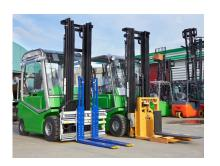
Electric forklifts do not impact indoor air quality. They are also quieter than non-electric lifts, allowing for improved communication and safer operation.
